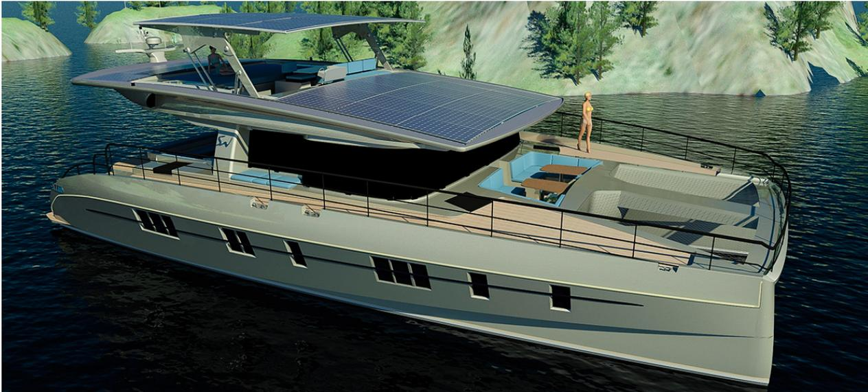
(<https://keyassets.timeincuk.net/inspirewp/live/wp-content/uploads/sites/18/2016/03/Solarwave-1-LEAD-IMAGE-flybridge-up.jpg>) Although it carries a diesel generator as a safety back-up (Solarwave quixotically refer to this as the ‘Range Extender’) the aptly named Solarwave 62’s vast 15kW solar panel array is designed to supply the boat’s entire electrical load on a day-to-day basis, motors and all.
