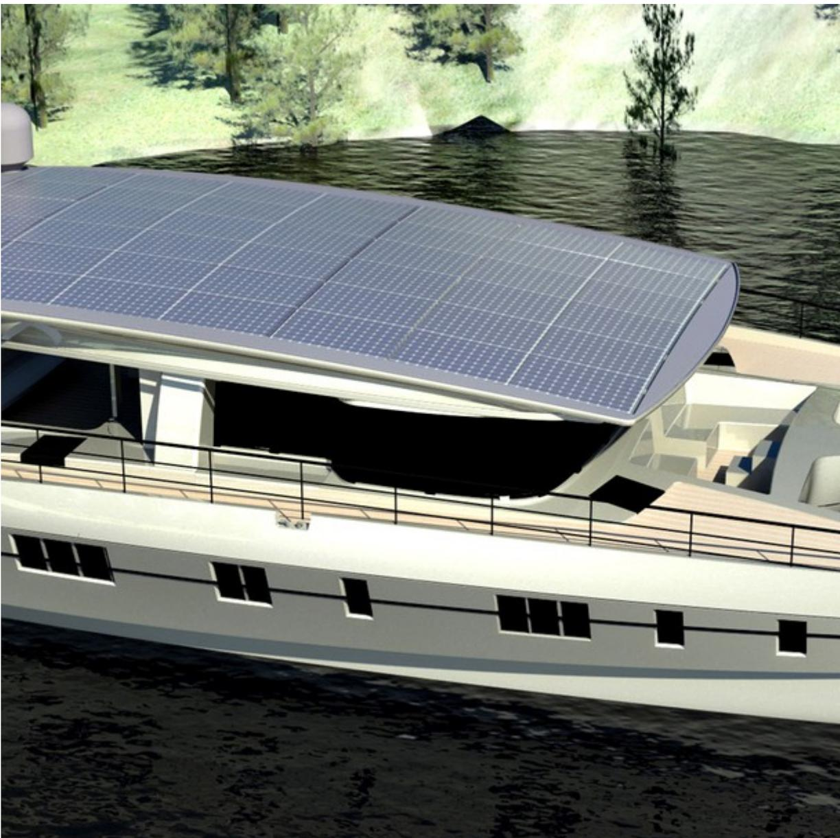
It's possible if you want. So they say at the Swiss company **Solarwave**, where they are manufacturing the first series of catamarans to run on solar energy. More specifically: their product is a **20-meter catamaran** that can be driven by electricity (provided by photo cells, with a generator installed as a reserve) or as a plug-in hybrid. The Solarwave Yacht has **68 square meters of solar cells** that charge two separate batteries with a **21% output**.
