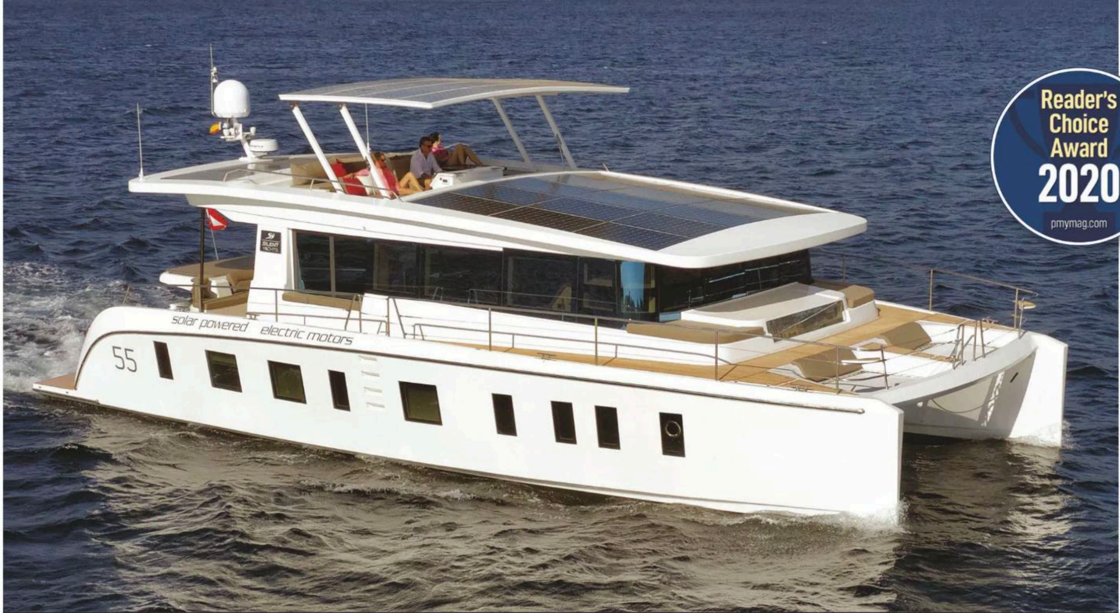
LOA 54'10" Beam 27'8" Draft 3'11" Displ. 38,000 lbs. Fuel 132 gal. Water 160 gal. Power 2/250-kW Dana TM4 E-motors Price $1.6 million
